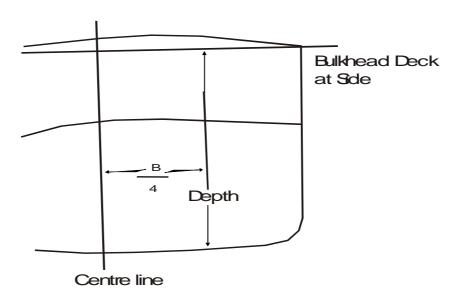
(4) The effective freeboard for each compartment shall be calculated from-
